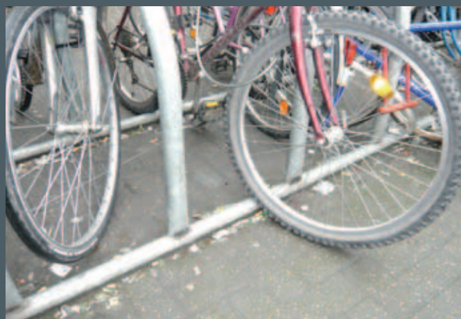
A good idea but bad in practice: a 'toast rack' with its stands too close together, leaving room for only one bike per stand. Note how the thick rail also traps litter
