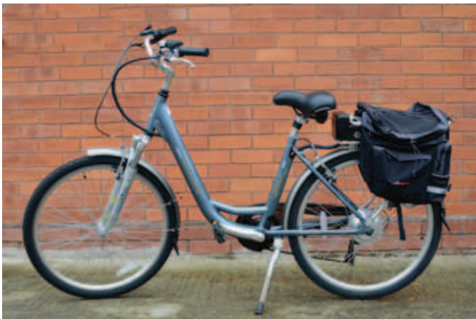
An electric cycle with the battery on the rear carrier and the motor in the hub of the rear wheel
